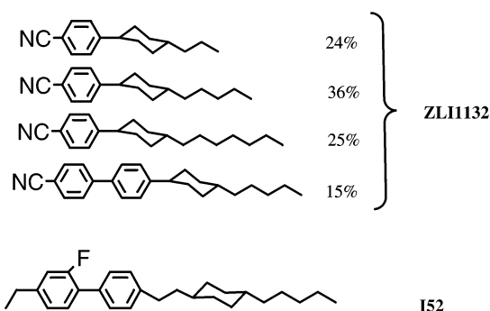
Figure 2. Structure and composition for the liquid crystals ZLI1132 and I52.
